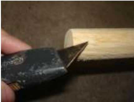
Trim both ends of the rattan with a utility knife
