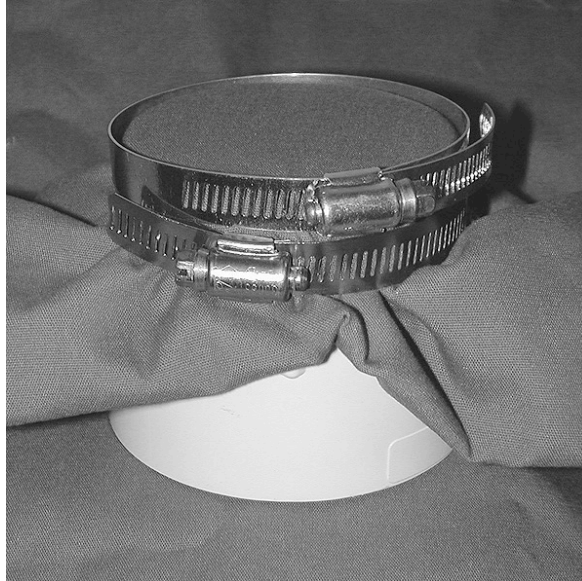
Figure 6 - Fabric clamped onto flange with two hose clamps. Notice that the second one will protrude a bit above the level of the fabric with thicker fabrics, but it should still be tight if you push everything down enough.
