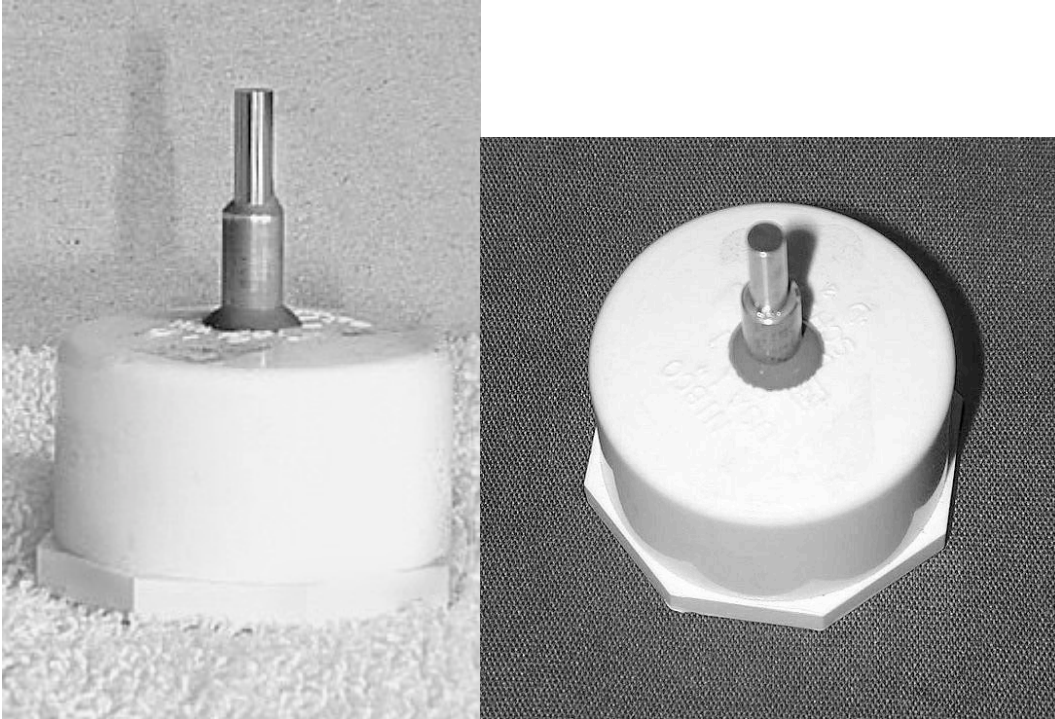
Figure 2 - Plastic cap with gage pin and drill collar sticking out, all epoxyed together (gray)
