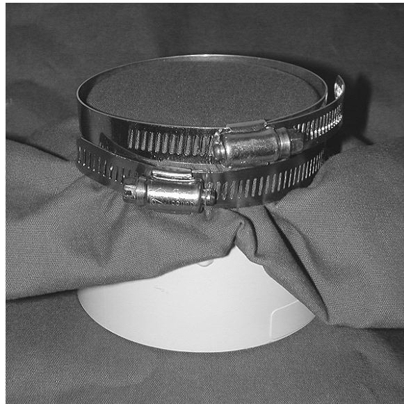
Figure 4 - Clamps and "frame" (3" flange) showing how these are assembled to carry out a fabric test.
